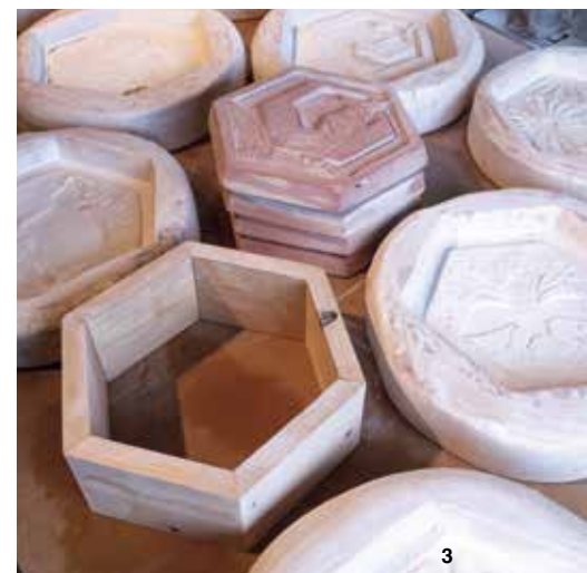
1 Eliane Medina, a Rat City Studios assistant, carving a paver model. 2 Jordan Jones, a visiting artist at Rat City Studios, carving a paver model. 3 The hexagonal wooden template that is used to create the original clay paver models, plaster molds of the carved paver models, and several pavers that were made from clay and glaze waste.
